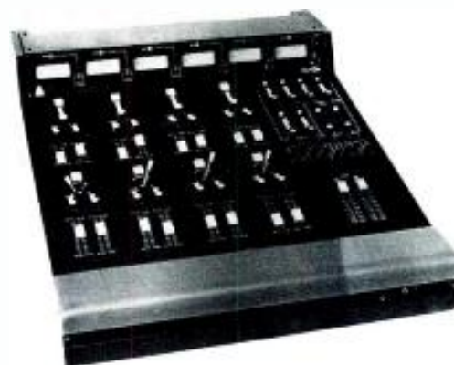
Panasonic's second-generation prototype Localization Processor. Once in production, the control section will be a considerably smaller package, with most of the electronics located in a remote rack mount location.
